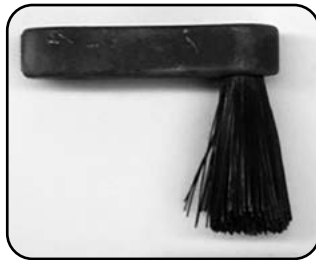
Level 2- Moderate splaying, have spare ready
